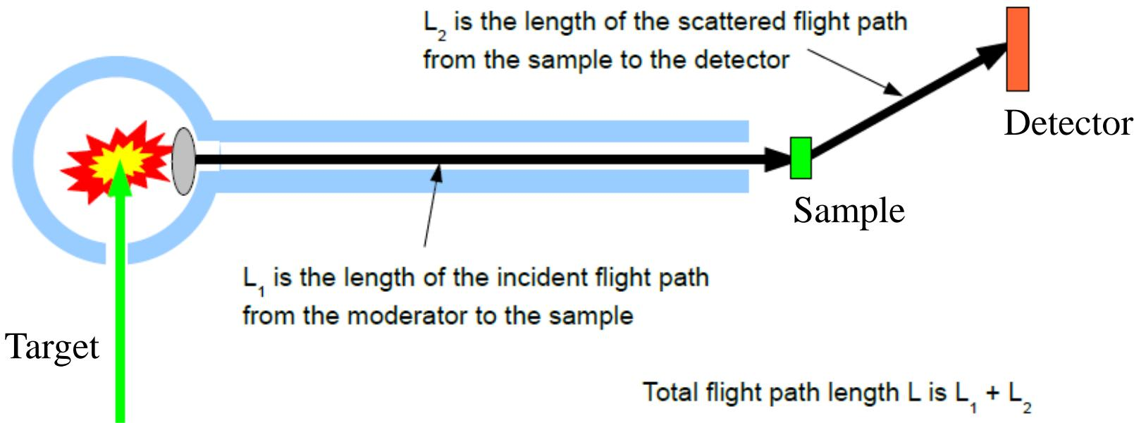
Sample irradiated by a pulsed neutron beam with wide range of wavelengths.
