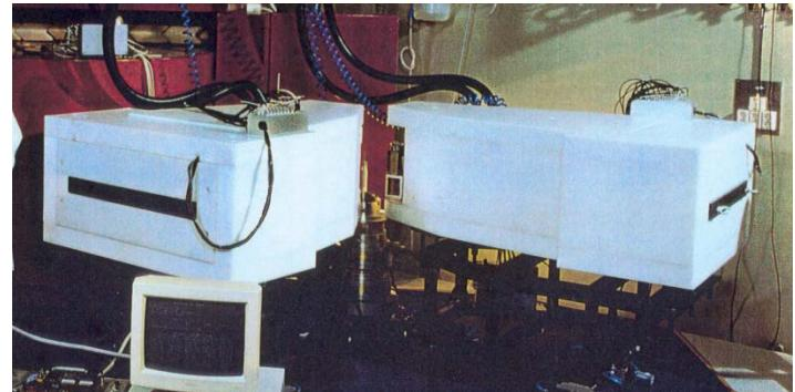
2 detector banks with 7 vertically stacked position sensitive detectors in each. Each bank cover 20° scattering angle.
