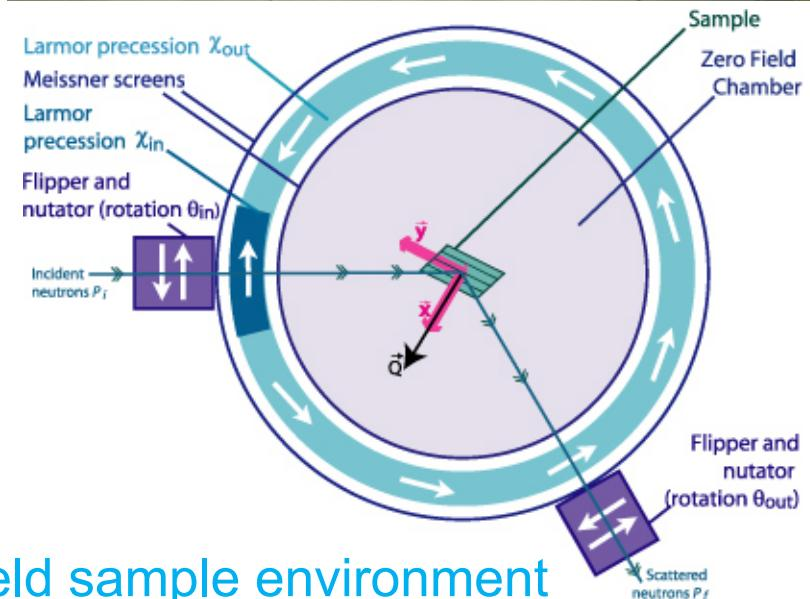
CryoPad: zero field sample environment
