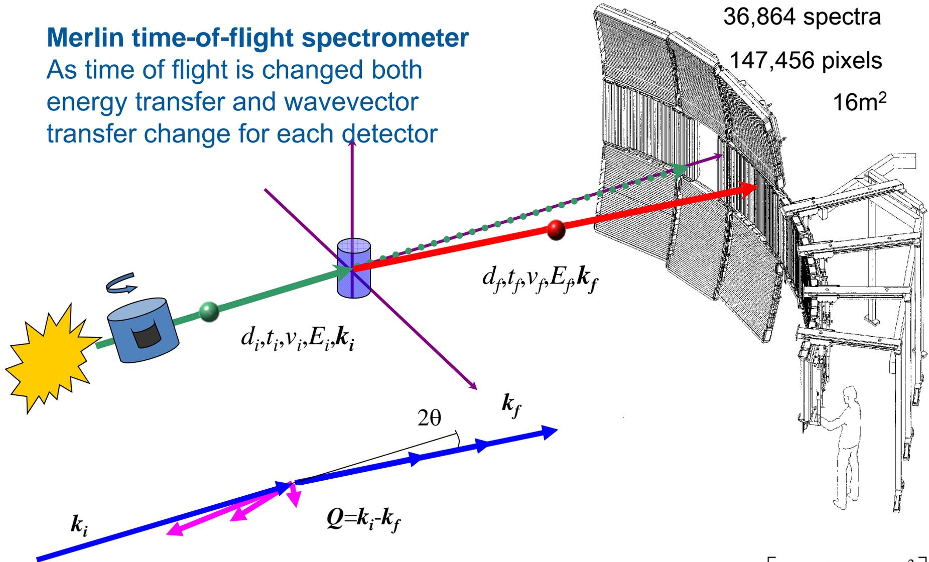
$$E = E_i - E_f = \frac{\hbar^2}{2m_n} (k_i^2 - k_f^2) = \frac{1}{2} m_n (v_i^2 - v_f^2) = \frac{1}{2} m_n \left[ \left( \frac{d_i}{t_i} \right)^2 - \left( \frac{d_f}{t_f} \right)^2 \right]$$
