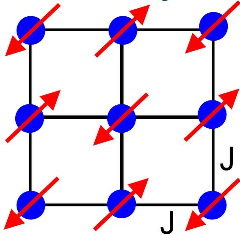
Anisotropy produces frustration if the anisotropy is incompatible with the spin direction favoured by the interactions
