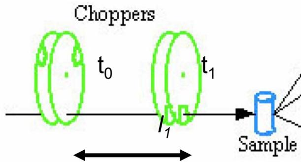
$$v_i = \frac{l_1}{(t_1 - t_0)}$$
