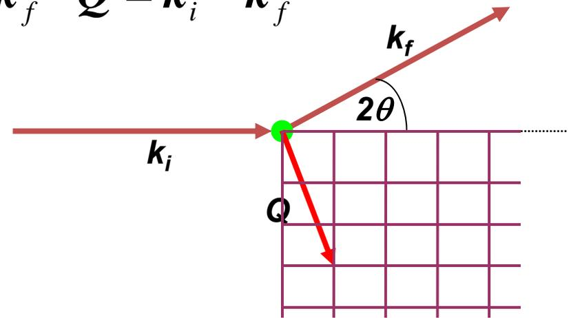
Scattering triangles - Inelastic  $\hbar\omega \neq 0; |k_i| \neq |k_f|$
