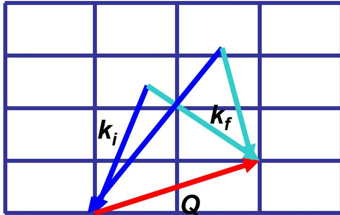
Keep energy transfer constant and, scan wavevector transfer.
